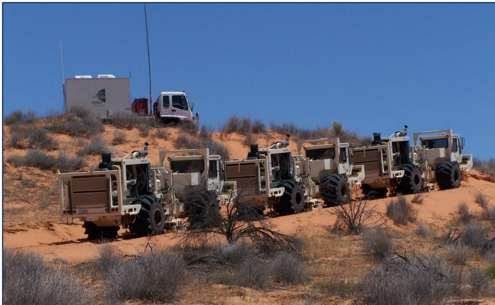
Figure 2: Vibroseis equipment used for onshore seismic data acquisition (Courtesy of Terrex Seismic)
