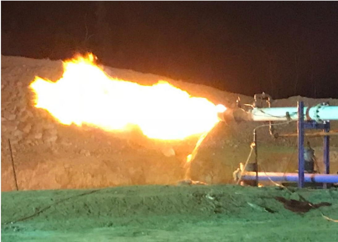
Figure 5 - Albany 1 flow test across a 13 metre interval in the Lake Galilee Sandstone Reservoir
